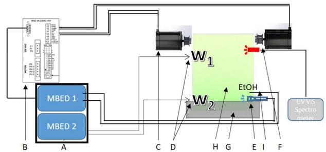
**Fig. 5** Diagram of the electronic control system. (A) is an electronic box with 2 MBED microcontrollers. The first one controls the variators (B) of the motors (C) and the photoconductive cells (E), the second one controls the humidity captors (D), placed respectively at the top and at the bottom of the film. (F) is the spectrometer, (G) is the tank, (H) represents a soap film. This scheme is not to scale
