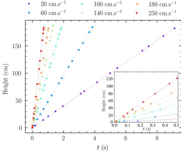
**Fig. 6** Altitude reached by the fishing line as a function of time. The dots represent measurements made with a high-speed camera with a frame rate equal to 125 for velocities between 20 and 140  $\text{cm s}^{-1}$ , and a frame rate equal to 250 for the velocities 180 and 250  $\text{cm s}^{-1}$ . The dotted lines correspond to the theoretical height  $V \times t$ . The inset is a zoom of this graph at short times, for  $t < 0.5$  s
