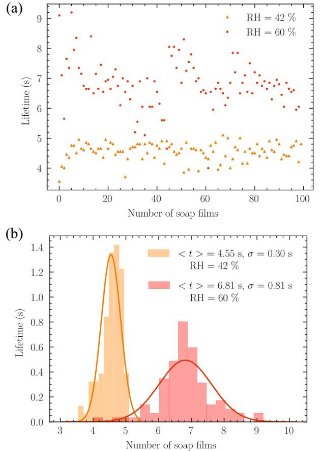
**Fig. 8** **a** Lifetime measurement of 100 soap films along an experiment performed at a velocity of 20  $\text{cm s}^{-1}$  with controlled humidities of 42% and 60%. The soap films break during their generation. **b** Histograms obtained for these two experiments. The lines represent the normal distribution
