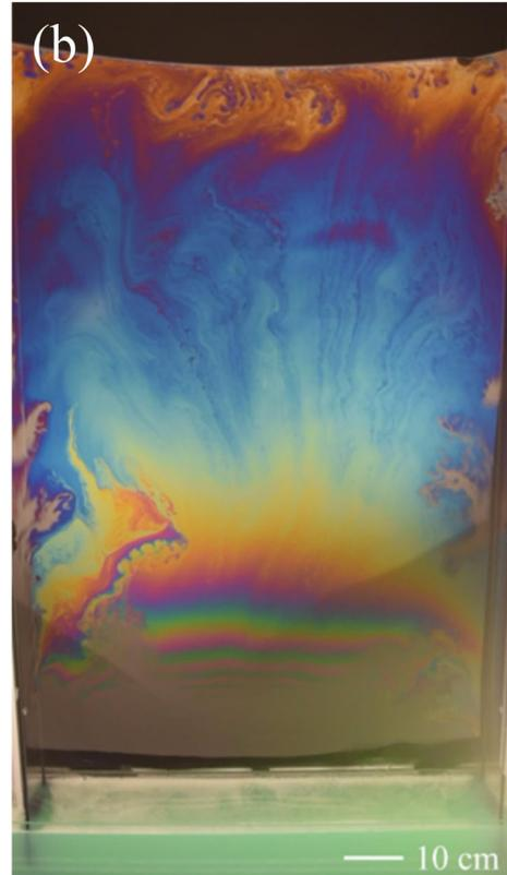
**Fig. 10** **a** Experimental setup used to visualize soap films. **b** Photograph obtained by using this set-up with a Nikon D7200 camera and a large angle objective lens. The film is generated at a velocity of  $50 \text{ cm s}^{-1}$  at a height of 120 cm with a 4% Fairy solution
