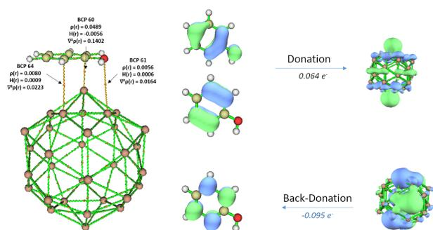
**Fig. 4** BCPs calculated within the QTAIM framework, along with the values of local properties, for flat configuration of phenol (left). The interacting molecular orbitals of phenol and GNP, as obtained within CDA framework (right).
