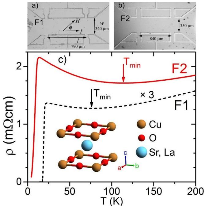
FIG. 1. Pictures of thin films (a) F1 and (b) F2, patterned by optical lithography. (c) Resistivity  $\rho$  of films F1 (dashed black curve, multiplied by 3) and F2 (solid red curve). Arrows indicate resistivity minima  $T_{min}$ . Inset shows the crystal structure of SLCO films.
