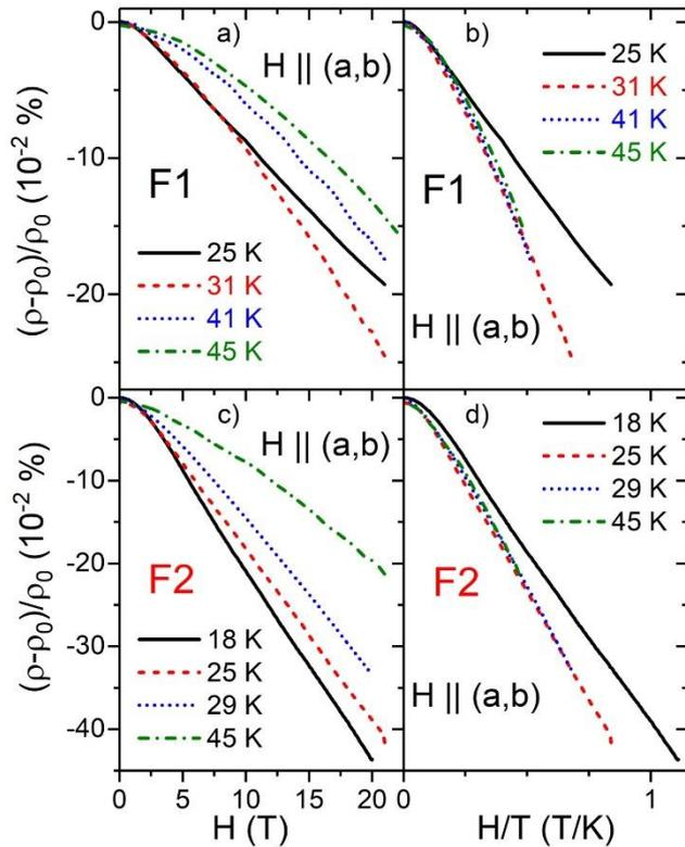
FIG. 2. (a) Normalized magnetoresistance  $(\rho - \rho_0)/\rho_0$  of F1 for magnetic field  $H$  parallel to  $\text{CuO}_2$  planes at different temperatures. (b) The same normalized MR as a function of  $H/T$ . (c) Normalized MR of F2 for magnetic field  $H$  parallel to  $\text{CuO}_2$  planes at different temperatures. (d) The same normalized MR as a function of  $H/T$ . The  $\rho_0$  is the zero-field resistivity, curves are smoothed, and measurement error is estimated to  $10^{-3}$  %.
