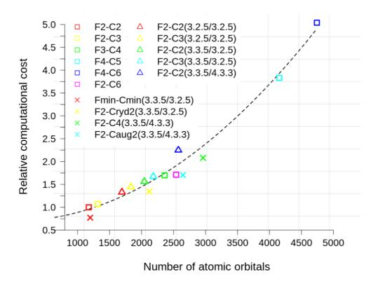
Figure 7: relative computational cost of RT-TD-ADFT simulations taking the F2-C2 basis set as reference. The dashed line is a parabolic fit over all data points. All the simulations have been run on the Adastra machine (CINES, France) with one node encompassing 8 GPU and 64 CPU.
