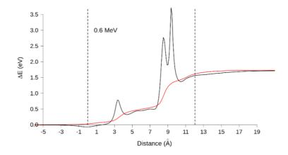
Figure 3: examples of energy profiles associated with the collision of a water slab by a 0.075 or 0.6 MeV proton. The black curve corresponds to the variation of ADFT energy ( $E^{ADFT}$ ) while the red curve corresponds to the variation of  $E^{mol}$  as a function of the distance of the projectile with the water slab. The vertical dashed lines indicate when the projectile enters and exits the van der Waals envelope of the water slab, the former instant defining null distance.
