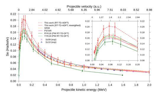
Figure 10: electronic stopping power obtained with our Gaussian Basis set RT-TD-ADFT approach using 29 QM/MM water cylinders. Comparison with experiments (Sz09 $^{62}$  and Sz10 $^{63}$ ), semi-empirical models (SRIM and PSTAR) and with other planewave (PW) RT-TD-DFT implementation of Reeves et al. (RYK16) $^{65}$  and Yao et al. (YYK19) $^{20}$ .
