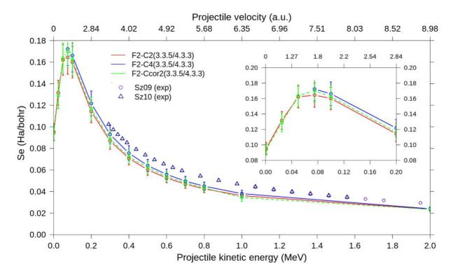
Figure 9: electronic stopping power obtained with our Gaussian Basis set RT-TD-ADFT approach using 20 QM/MM water cylinders. Comparison with experiments ( $Sz09^{62}$  and  $Sz10^{63}$ ). Three basis sets are tested.
