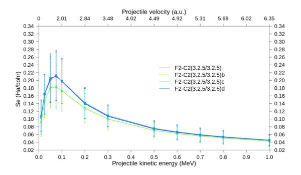
Figure 6: electronic stopping power for proton in water slabs as a function of the projectile kinetic energy with a Dunning standard basis set augmented by AOC placed on various atoms (see Table 2). The error bars are the standard deviations calculated over the 12 water slabs with a confidence interval of 95%.
