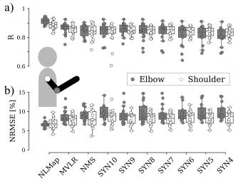
Fig. 6: **Multi-joint model accuracy.** In both panels, data for the elbow joint is represented in gray, and data for the shoulder joint in white. a) Pearson's correlation coefficient b) Normalized root mean square error
