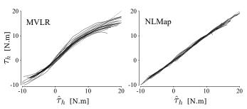
Fig. 7: **Effect of mapping nonlinearization on Elbow torques.** Comparison between MVLR and NLMap of reference  $(\tau_h)$  to estimated  $(\hat{\tau}_h)$  torques correlations. Each line corresponds to one participant and represents the smoothed data from the ten 30s trials.
