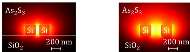
Fig. 2. Views of two different hybrid slot waveguides characterized by 70\text{nm} and 200\text{nm} slot widths, respectively.
