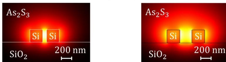
Fig. 2. Views of two different hybrid slot waveguides characterized by 70nm and 200nm slot widths, respectively.
