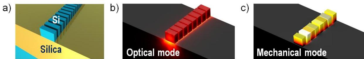
Fig. 1. (a) Schematic view of the proposed optomechanical silicon waveguide exploiting subwavelength periodic structuration. Calculated (b) optical and (c) mechanical modes of the subwavelength silicon waveguide.
